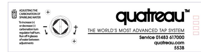
The CO2 is controlled via the gas canister regulator on the front of the unit (see diagram).
