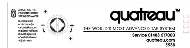
The CO<sub>2</sub> is controlled via the gas canister regulator on the front of the unit (see diagram).
